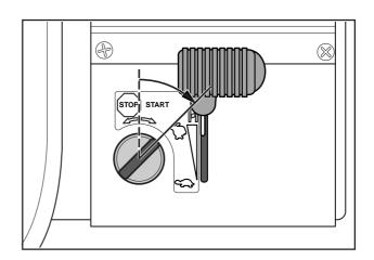
**7.** When the engine has started release the ignition key to neutral position.
